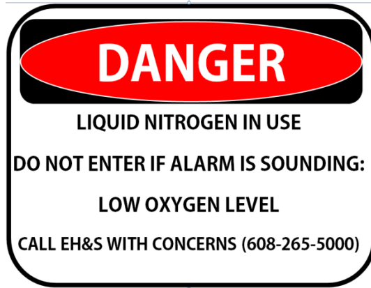
Figure 2: Example sign posting for Level 3 and 4 facilities
